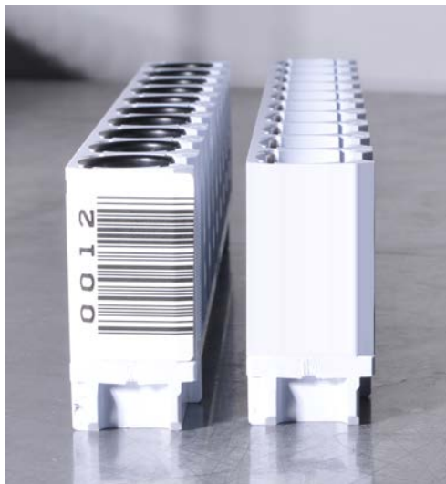
Figure 6.70 Rack ID Label on a Rack
